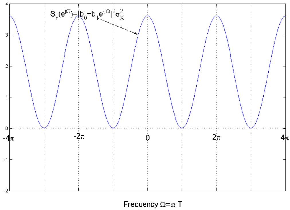
Figure 6: Power spectrum of filtered white noise
