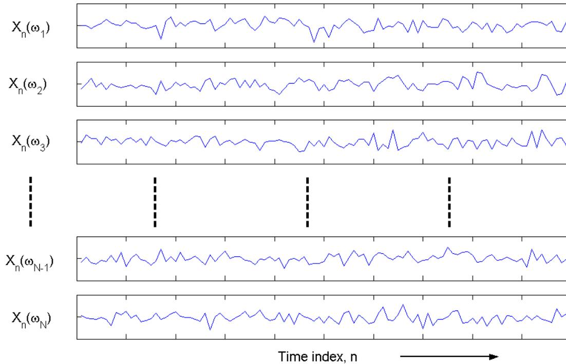
Figure 1: Ensemble representation of a discrete-time random process
