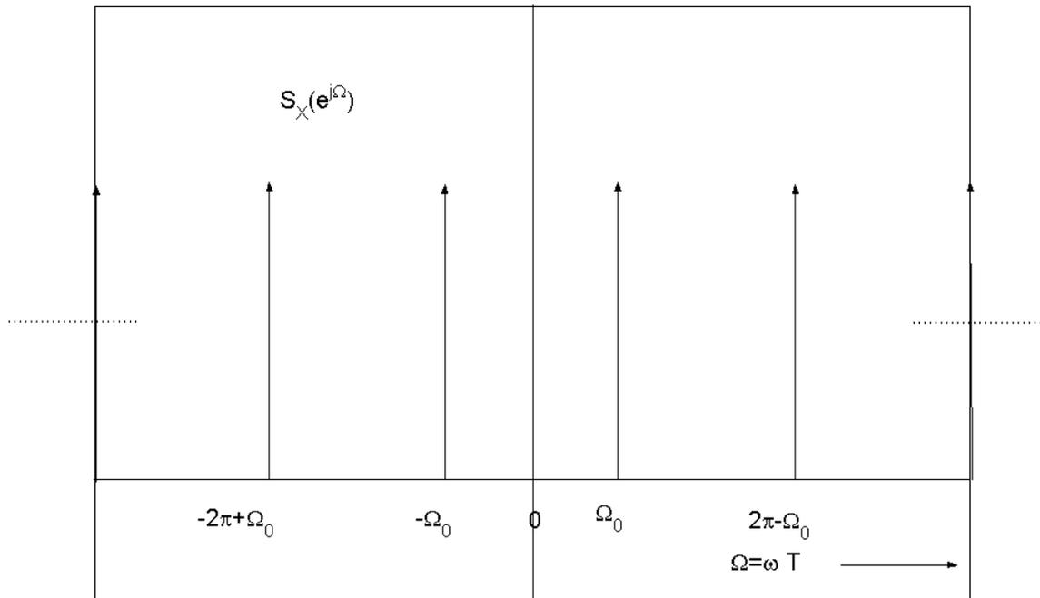
Figure 3: Power spectrum of harmonic process
