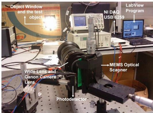
Fig. 1. System setup.
