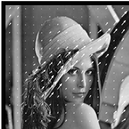
Fig. 6. ICP shift independence: the input image of figure 5b has been shifted by half a sample in each direction prior to ICP transform. Although this shift corresponds to the worst alignment case, we observe minor changes in the ICP coefficients.
