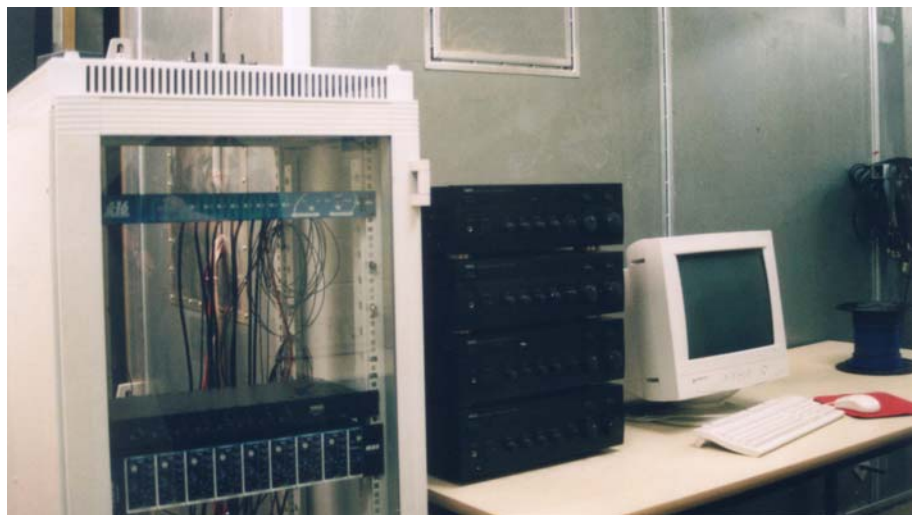
Figure B.7: Photograph of the equipment used to drive the speakers.
