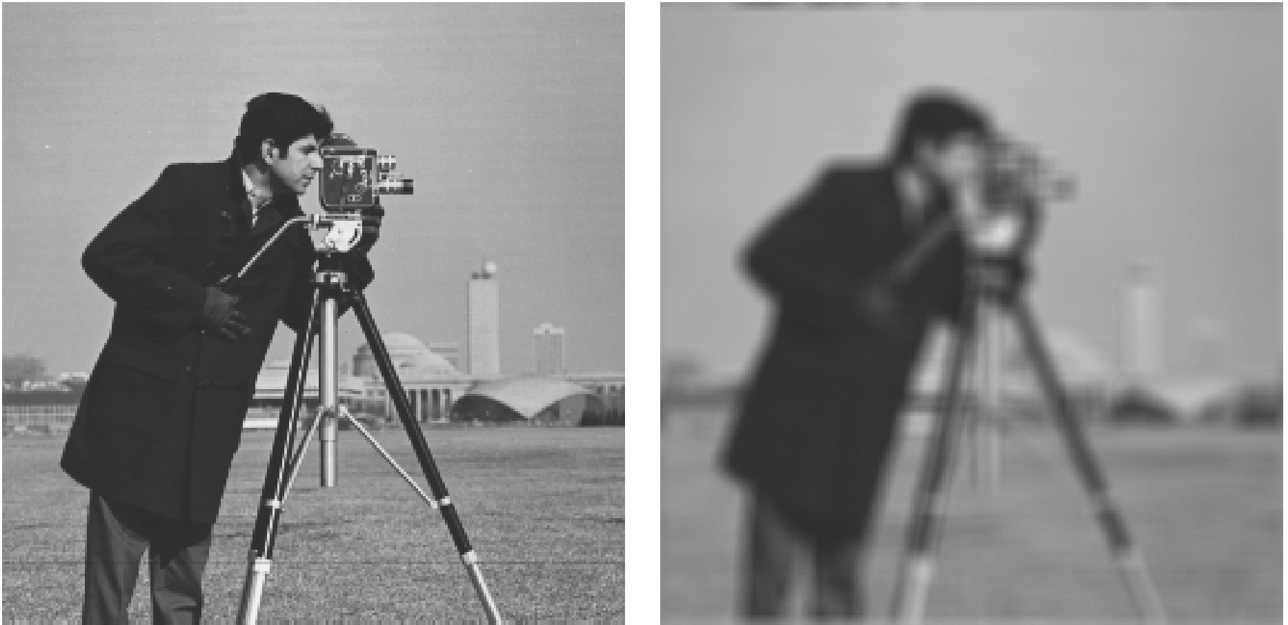
Figure 5: Original Cameraman image (left) and version (right) blurred with a 9 \times 9 uniform filter H plus added white Gaussian noise of \sigma = 0.555 (BSNR = 40 dB).
