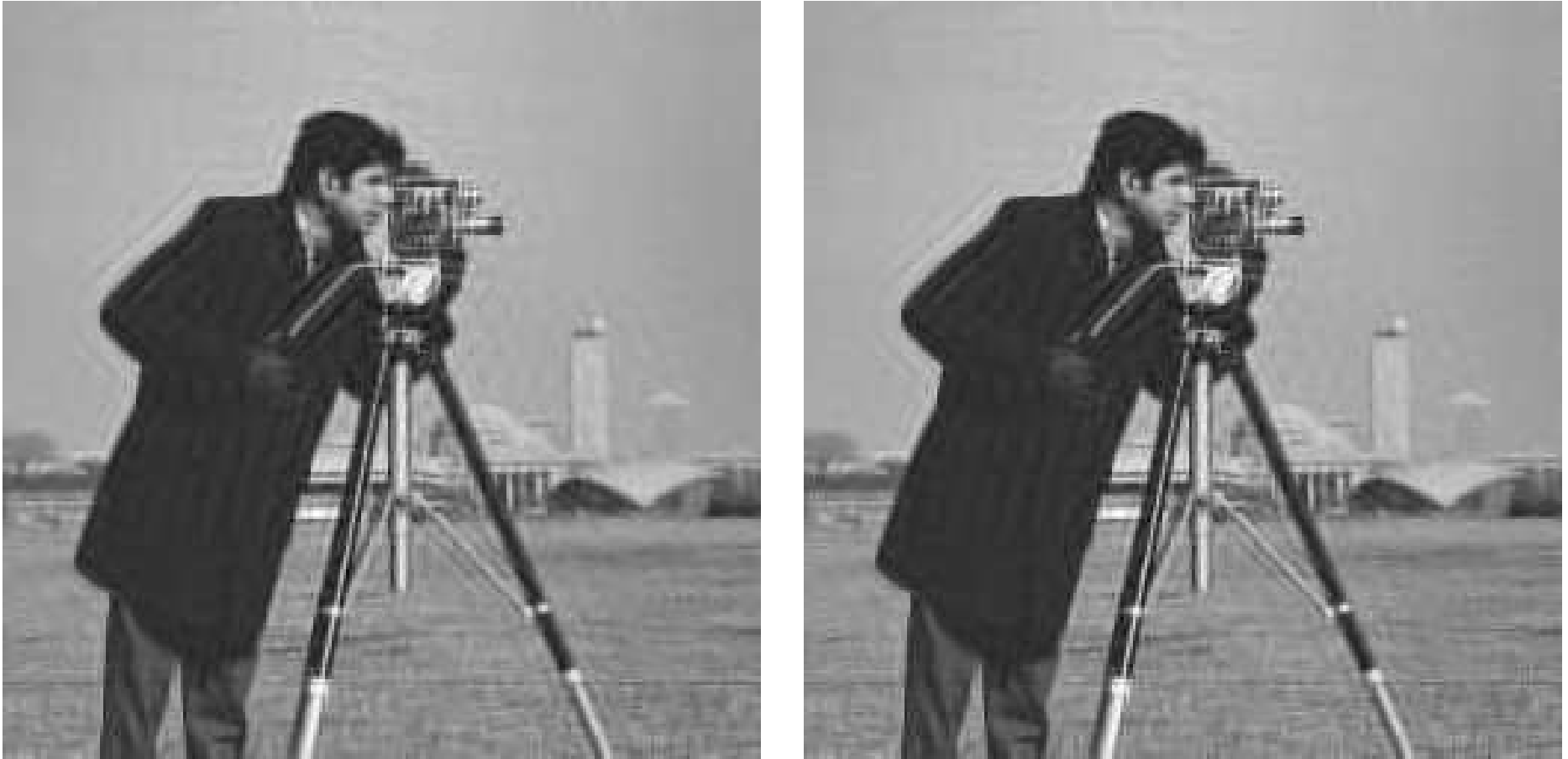
Figure 9: Output images after iterations 1 (left) and 4 (right) of the Conjugate Gradient algorithm. \text{ISNR} = 7.22 and 7.57 dB respectively.
